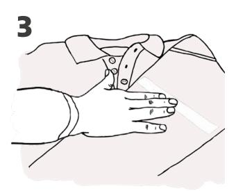
Place the reflective film on the substrate with the adhesive side down. Avoid applying the film over seams and stitches.
