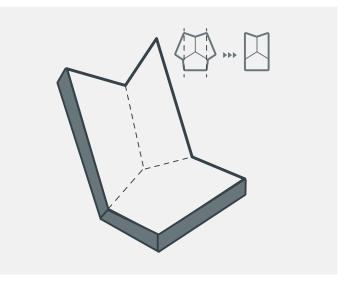
The incident light is lost in the corners. (triangular angle reflector, tetrahedron shape)
