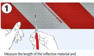
Measure the length of the reflective material and cut from the roll.
