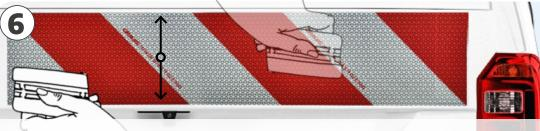
Even out with squeegee from centre to edge to remove uneven parts and air pockets.
