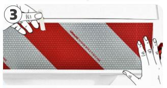
Position the sheeting on the vehicle – tape strips might help to hold it in place. Press the part without carrier film onto the surface using a squeegee.
